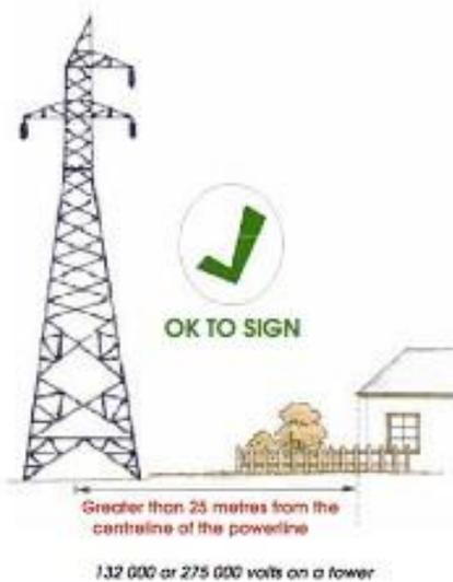
Transmission lines are very high voltage powerlines that carry electricity from power stations to major substations, or between major substations. These are normally seen in country areas or on the outskirts of towns.
